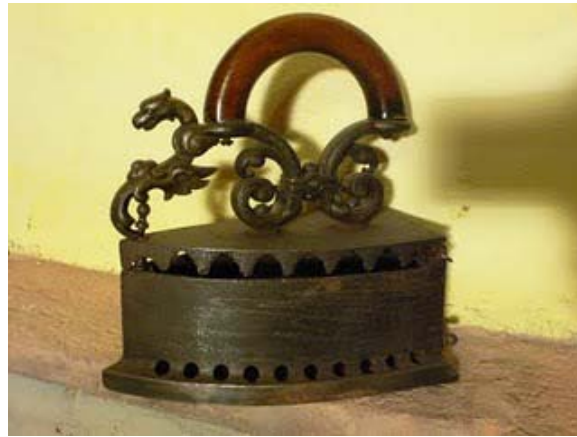
Cast-iron ironer, operated with coal
